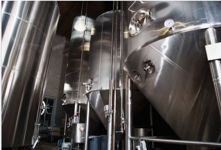
Image 1. Brewery fermentation tanks. Though this is not exact to the infrastructure needs of SCP production, fermentation tanks are a component to their upstream production processes.
